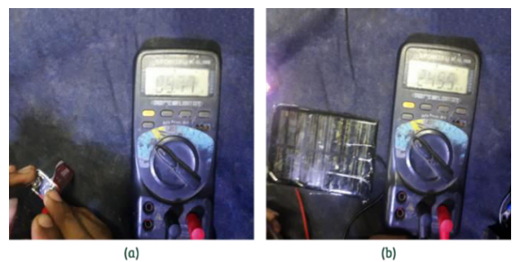
Fig. 8: (a) Voltage measurements of a 12V dry cell, and (b) Voltage measurements of a solar panel.
