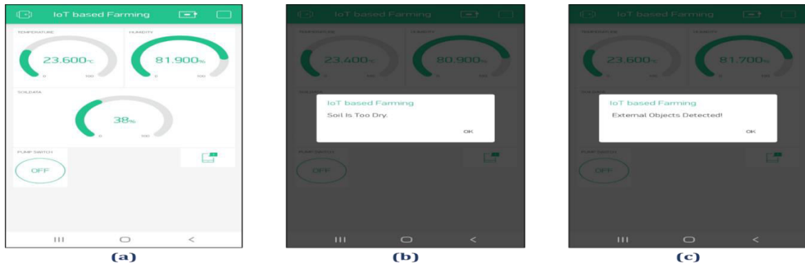
Fig. 15: (a) Blynk software interface, (b) Notification when soil is dry, and (c) Notification when external object detect.
